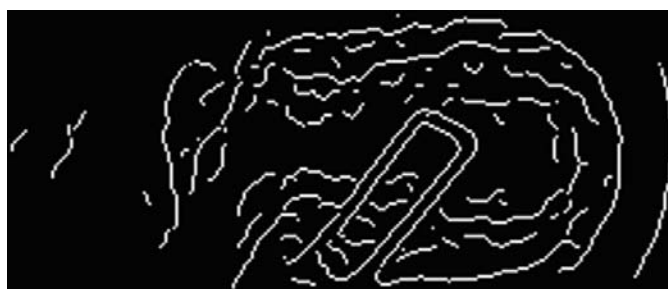
Figure 3 Canny edge-detection is a very sensitive method to extract crystal edges and gradient orientations. It is obvious that strong object selection must be applied to remove the numerous artifacts created by this method. Subsequent processing will detect the lines among all the selected skeletons.
